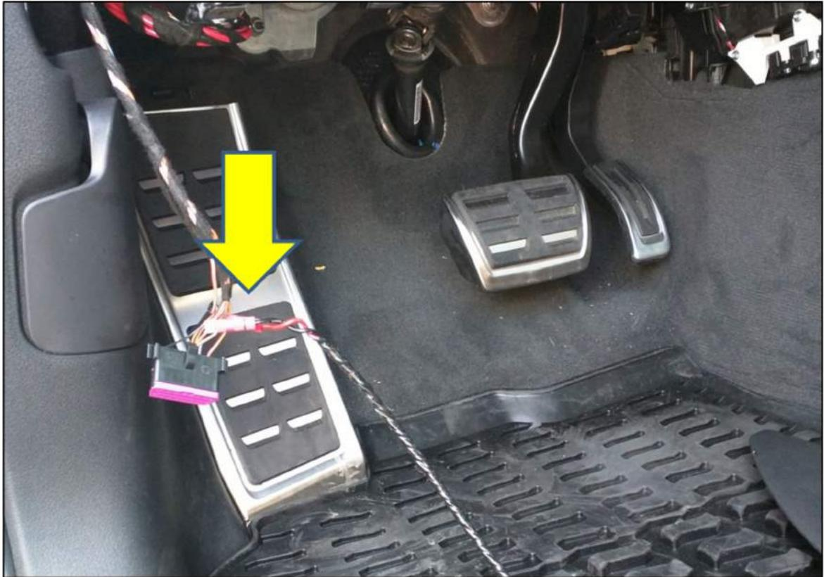
In this picture we can see that the 12V and Ground connections have been made using the recommended Posi-Tap connectors.
