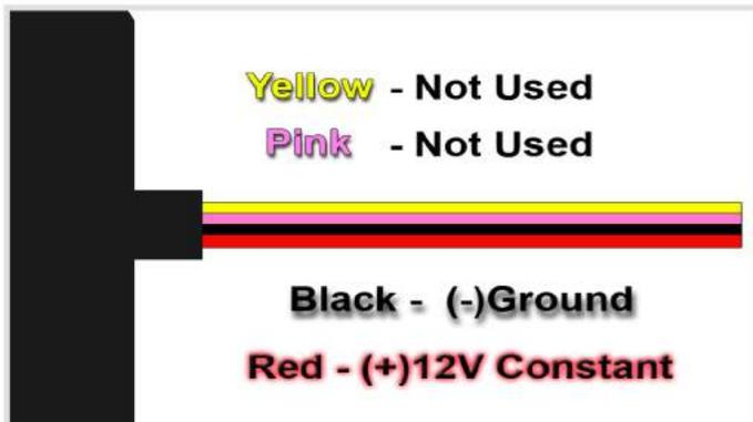
After you have found a suitable place to mount the device you will want to cut your excess wire and make the necessary electrical connections to power the unit.
