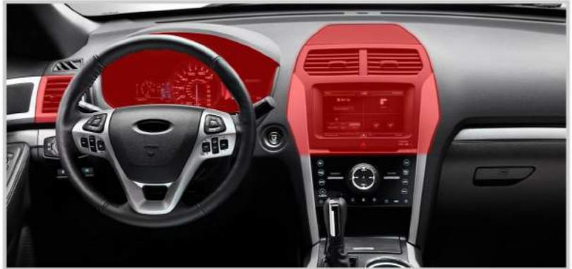
When mounting the Trax device, the LED's *must* be facing up and the device should not be obstructed by metal.
